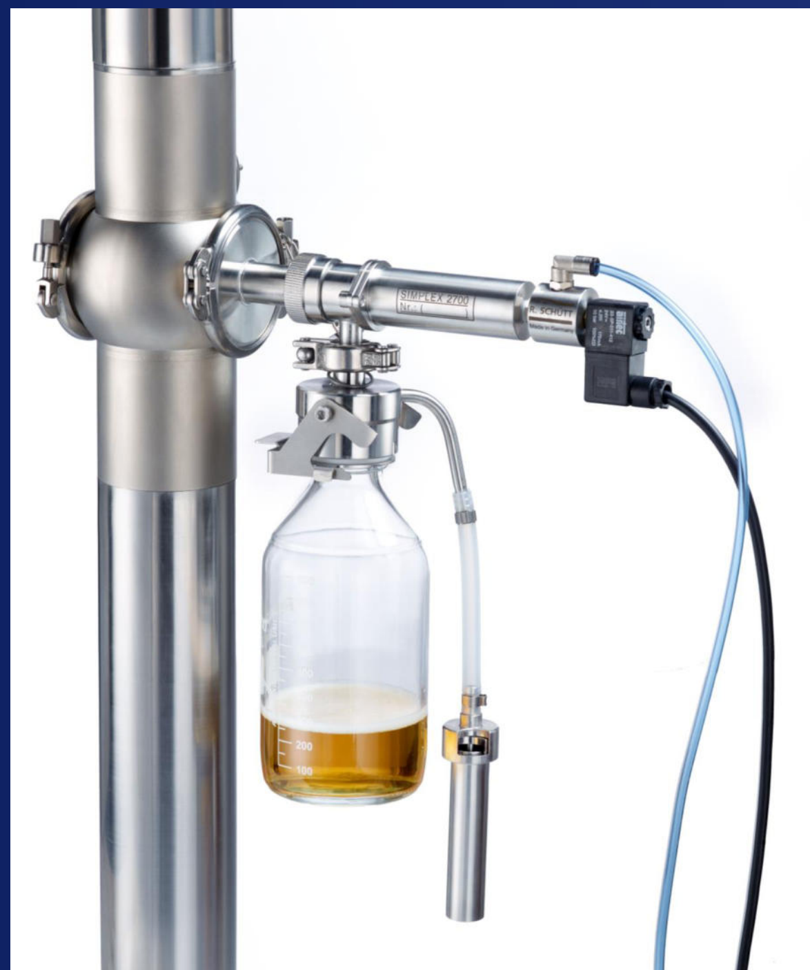
Simplex 2700 with attached 3/2-way pneumatic valve.
