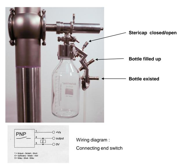
End switch (optional) is adjust optimally.
