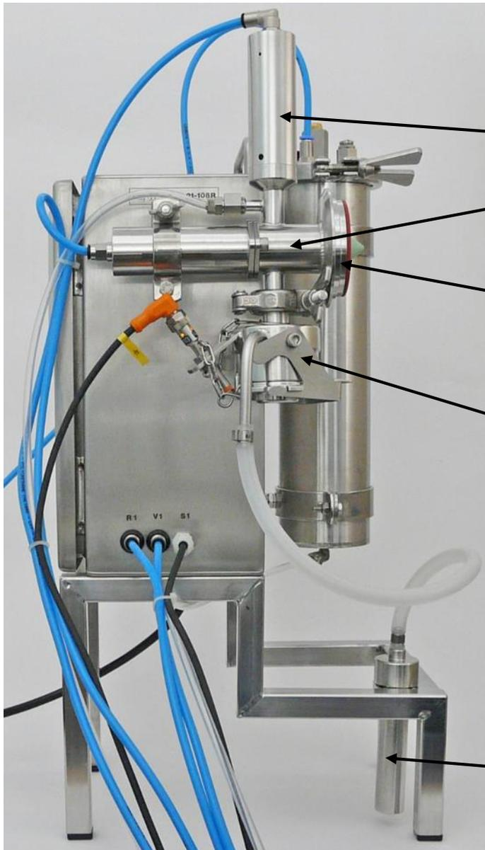
The illustration shows the cleaning valve in use on a portable system.
