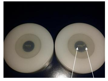
If the slit in the membran is not ok you can get a microbilogical probelm. You can recognize it by the form of the slit.
