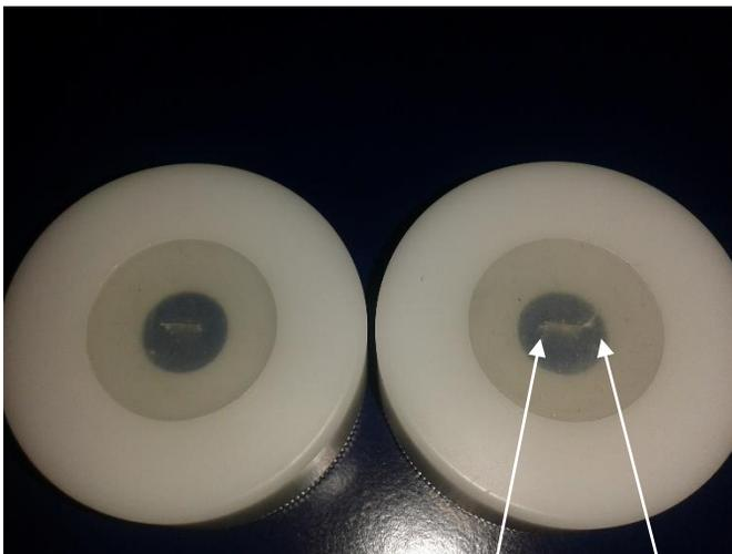
If the slit in the membran is not ok you can get a microbiological problem. You can recognize it by the form of the slit. If rips arise at the ends of the slit, it's very important to change the membran.
