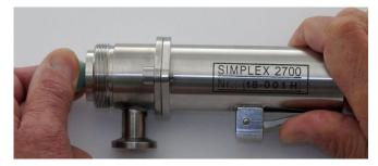
**2. Step** Push the hand lever and screw out the spindle with seal cone
